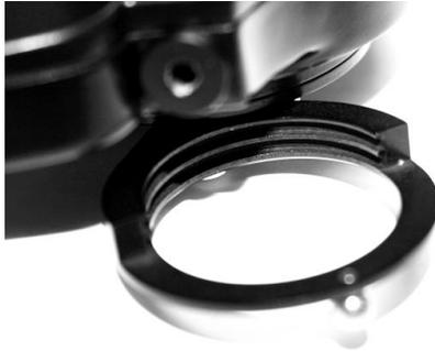
**Please note:** For models that have LED illumination, an additional swing-out filter carrier is provided. LED illumination provides a very white light that needs to be softened with a neutral diffusing filter when using the 10X objective. Place the neutral diffusing filter in the secondary filter carrier. Rotate the disc to the desired phase magnification (10, 20/40, or 100) to match the objective you are using. (Please note: the 4x objective included with the system is **not** phase)
